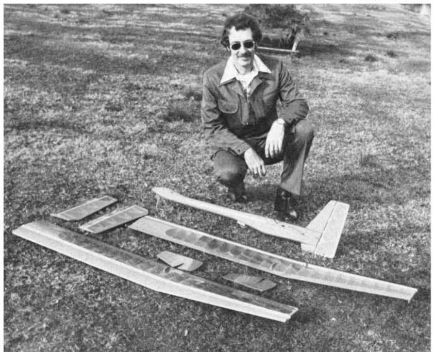
It collapses whenever you want. Also depending upon the fortunes of flight. Wing panels pull, as do the tail surfaces for cramming into compact sized vehicles. A stimulating new concept in R/C.
